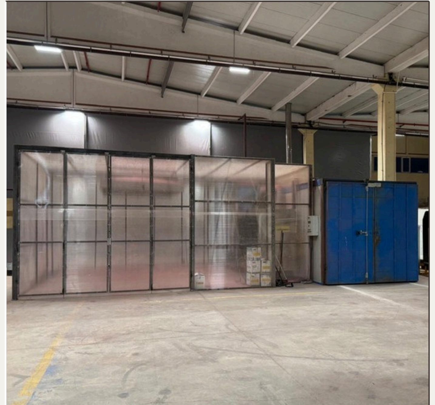
Powder Coating Unit for High-Volume Products, measuring 8m x 3m x 3m.
