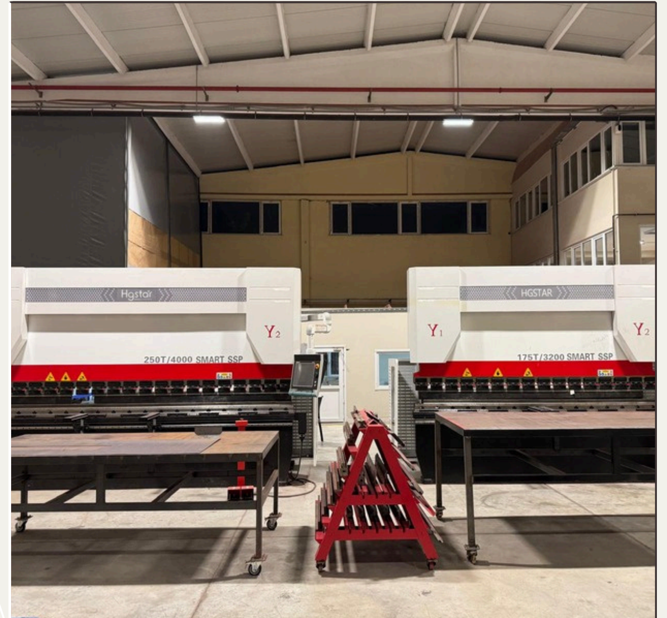
CNC BENDING COMPONENTS 4000 mm 250 tons 3200 mm 175 tons
